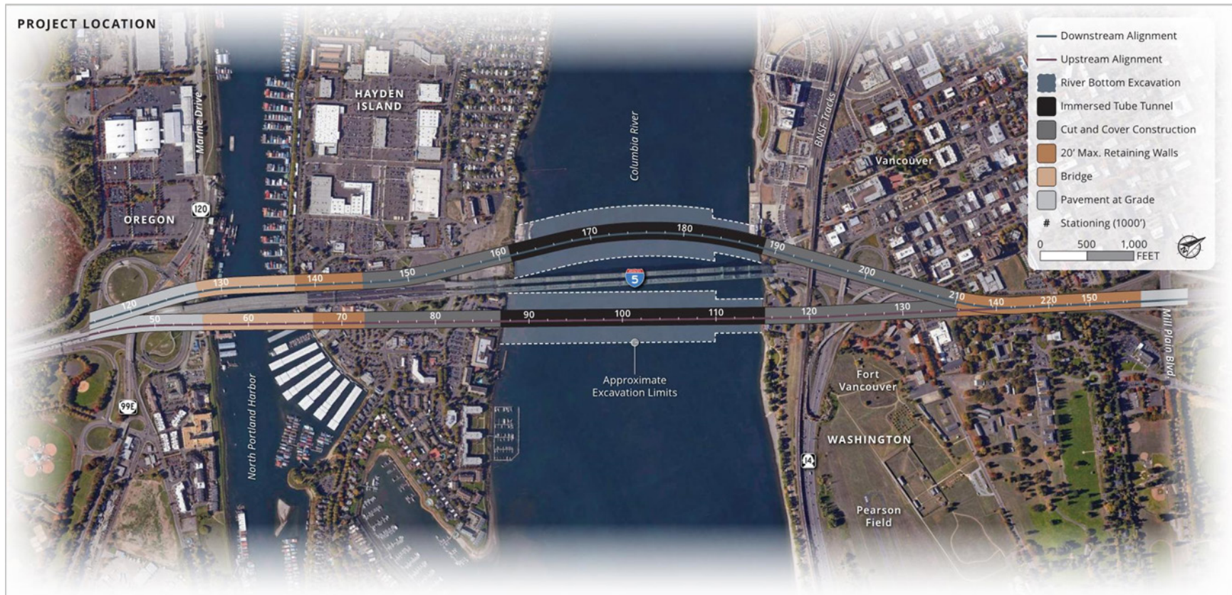
Figure 2. Upstream and Downstream Tunnel Alignments
